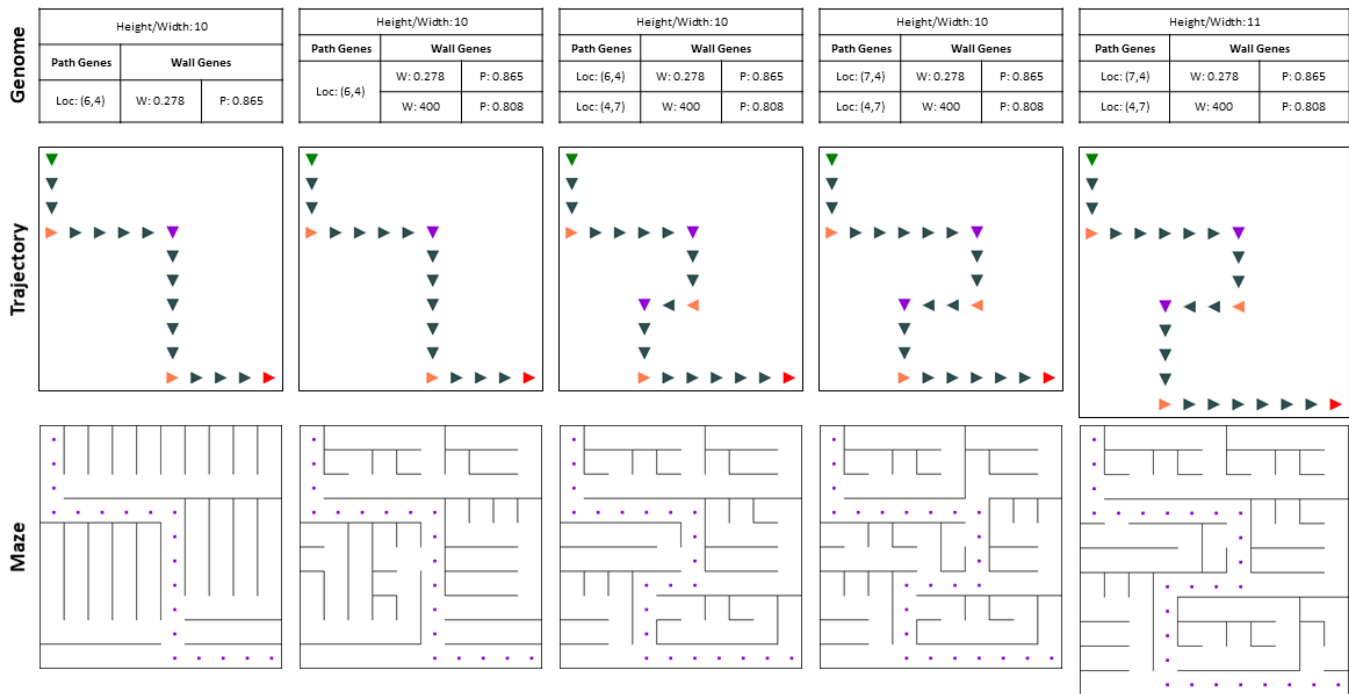
Figure 2: The maze evolution process. Maze genotypes (top), respective trajectories (middle), and respective phenotypes (bottom) are shown. The table above each maze enumerates the path (waypoint) and wall genes, while the visualization directly below depicts the resulting trajectory. In the maze phenotypes at bottom, dots are shown to depict the solution path. Each path gene specifies the coordinates of a waypoint, and each wall gene contains a wall position and passage position, both real numbers in the interval [0, 1] . The wall position (W) describes the relative position of a wall within a sub-space induced by the solution path, while the passage position (P) describes the relative position of a passage (opening) within that wall. The initial genome (first column) consists of one path gene and one wall gene; the single wall gene is repeated to fill out all sub-spaces. The second column depicts an add wall mutation, while the third column demonstrates an add waypoint mutation. In the fourth column, a mutate waypoint operation is carried out, shifting the first waypoint one unit to the right. Finally, the fifth column depicts an expand maze mutation, extending the outer boundaries down and to the right, and resulting in a corresponding extension of the solution path.
