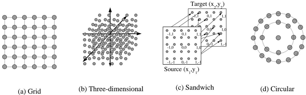
**Figure 6: Alternative Substrate Configurations.** This figure shows (b) a three-dimensional configuration of nodes centered at  $(0, 0, 0)$ , (c) a “state-space sandwich” configuration in which a source sheet of neurons connects directly to a target sheet, and (d) a circular configuration. Different configurations are likely suited to problems with different geometric properties.
