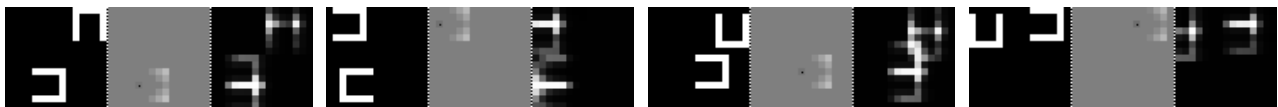
Figure 10: Trial images for a run using the Cs library. The left part of a trial image shows the input to the network, the middle part shows the weight values from all input neurons to the single output neuron corresponding to the centre of the target shape, and the right part shows the output of the network (50% grey represents zero weight, black represents a maximum negative weight value, white represents a maximum positive weight value, a black dot indicates a negative value). The same weight pattern is reproduced over four output neurons in different positions. The weight pattern produces maximal output for the target shape only.
